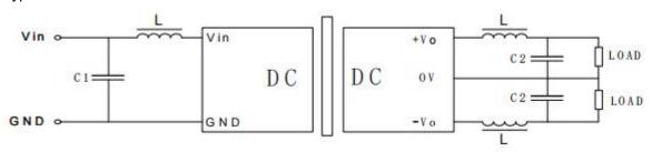
Note 2: C1 is 4.7uF/50V, LDM is 6.8uH, Cout is 10uF/50V
